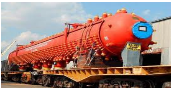
Fig 5. Transportation of boiler drum
