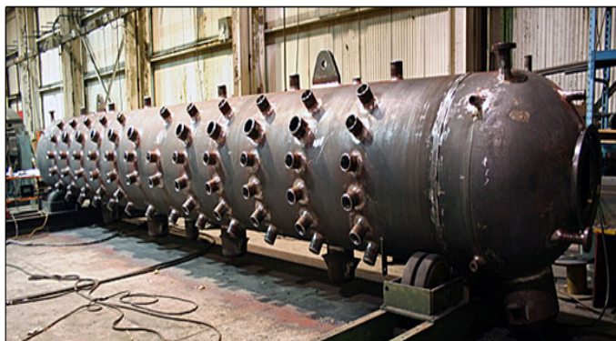
Fig.4 Manufacture of Boiler drum
